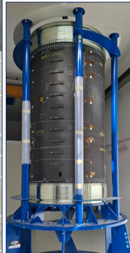
Cryotank static load test
