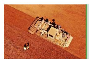
Mining applications are in continuous improvement. A range of new materials like pozzolan are now being mined with Surface Miners
